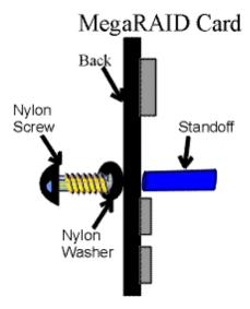
Insert the large 4-40 nylon screw through the nylon washer and through the mounting hole on the MegaRAID Card, starting from the back of the MegaRAID card.
